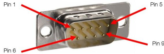
Figure 174 - DE9 Male connector (Pin side view)
