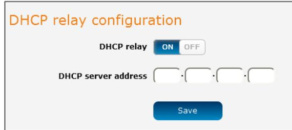
The screenshot shows the 'DHCP relay configuration' window. At the top, the title 'DHCP relay configuration' is displayed in orange. Below the title, there is a 'DHCP relay' toggle switch currently set to 'ON'. Underneath, the 'DHCP server address' field is represented by four empty input boxes separated by dots. At the bottom of the window is a blue 'Save' button.
