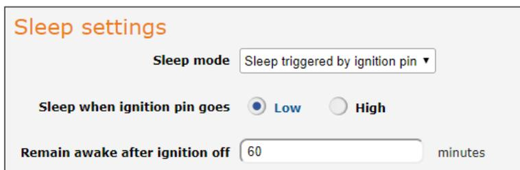
The screenshot shows the 'Sleep settings' section with the 'Sleep mode' dropdown set to 'Sleep triggered by ignition pin'. Below it, there are two radio buttons: 'Low' (selected) and 'High'. At the bottom, the 'Remain awake after ignition off' field contains the number '60' and is followed by the text 'minutes'.
