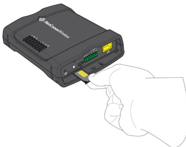
Figure 17 – Inserting the SIM card
