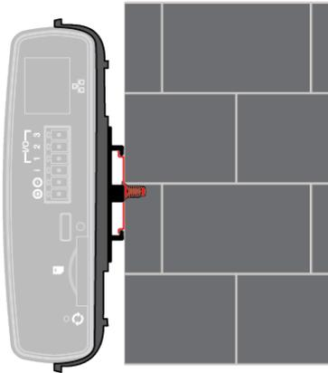
*Figure 9 – Wall mount with DIN rail mount adapter*
