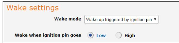
The screenshot shows a configuration panel titled "Wake settings". It contains a "Wake mode" dropdown menu set to "Wake up triggered by ignition pin". Below this is a "Wake when ignition pin goes" section with two radio buttons: "Low" (selected) and "High".
